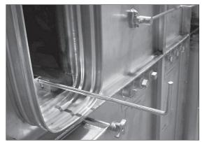
Prefilter Removal Rod Shown Partially Extended
