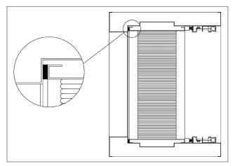
BG-Series and KG-Series Filter Locking Mechanism
