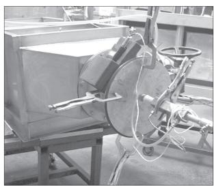
Pressure Decay Leak Testing of a BG-Series Containment System
