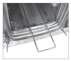
Primary Filter Removal Rod Shown Partially Extended
