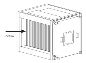
**Right-Hand Access:** Looking in the direction of air flow from the upstream side of the housing with the door on your right, the unit is right-hand access.
