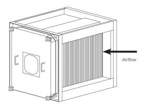
**Left-Hand Access:** Looking in the direction of air flow from the upstream side of the housing with the door on your left, the unit is left-hand access.
