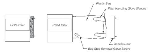
2. Carefully draw contaminated filter into bag and place filter (in bag) on stand or table. Remove arms from bag. Seal bag between access port and filter. Cut bag, leaving bag stub attached to access port. Place new filter into a new bag. Place new bag over bag stub attached to access port.
